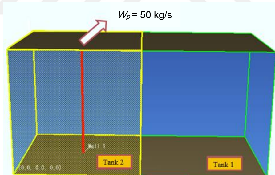
Figure 3.22 : Modelling of two tanks production case with PETRASIM.
