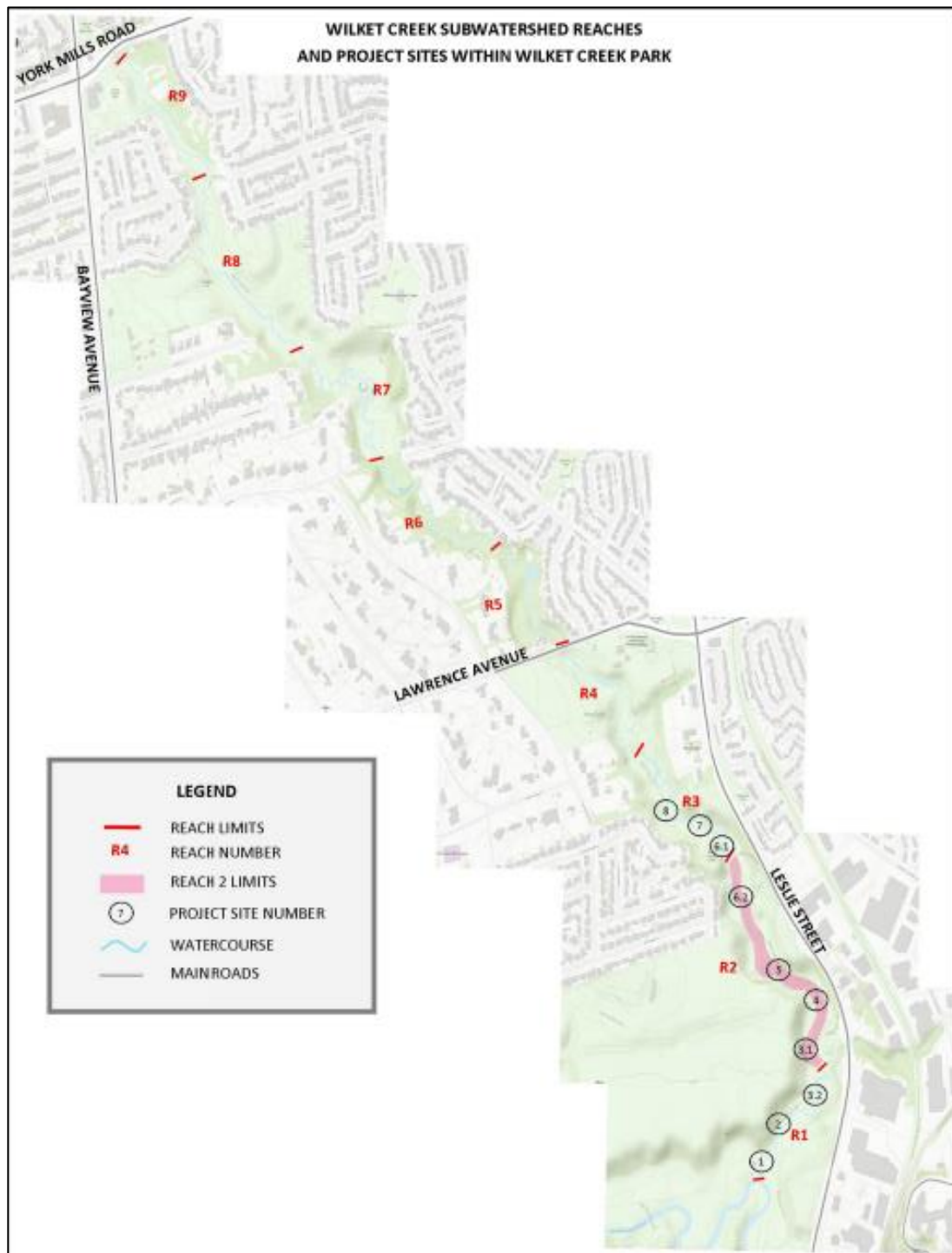
Figure 4.4: The restoration sites as defined by the Wilket Creek Channel within Wilket Creek Park Rehabilitation Study and Geomorphic Systems and Habitat Study. Emergency works to reconstruct the channel and protect surrounding infrastructure at project sites 2, 3.1, 3.2, and 7 was completed between April 2011 and fall 2015. The two reaches highlighted are the two discussed above in Section 3.5 (modified from Parish Aquatic Services, 2014)
