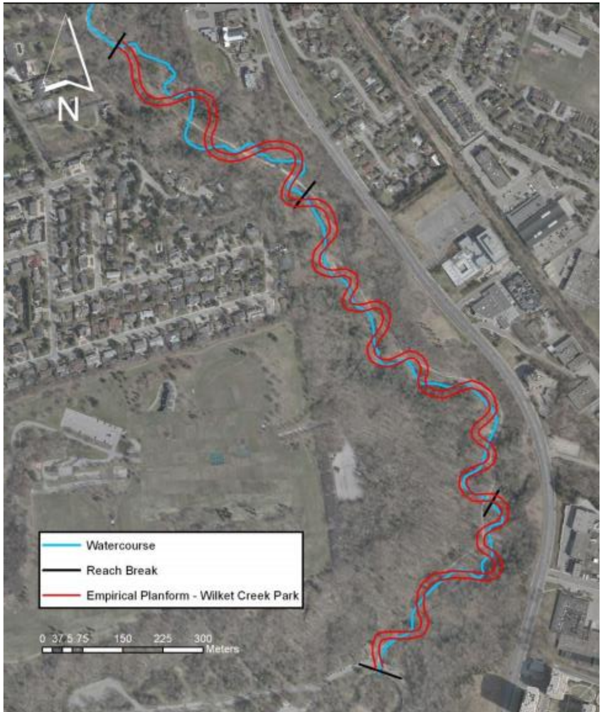
Figure 4.5: The current planform of Wilket Creek's watercourse (blue) south of Lawrence Ave E. This is compared to the empirically designed proposed planform
