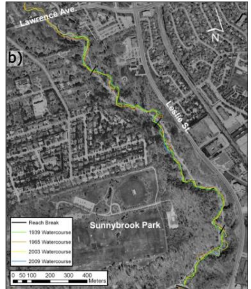
Figure 3.29: The planform alignment of a) the upstream reach and b) the downstream reach of Wilket Creek. The planform in b) begins before the beginning of urbanization while the planform in a) begins during urbanization. The greatest change in planform morphology is between 2009 and 2013. This may be due to further reconstruction after a flood event in 2005 (modified from Parish Aquatic Services, 2013).
