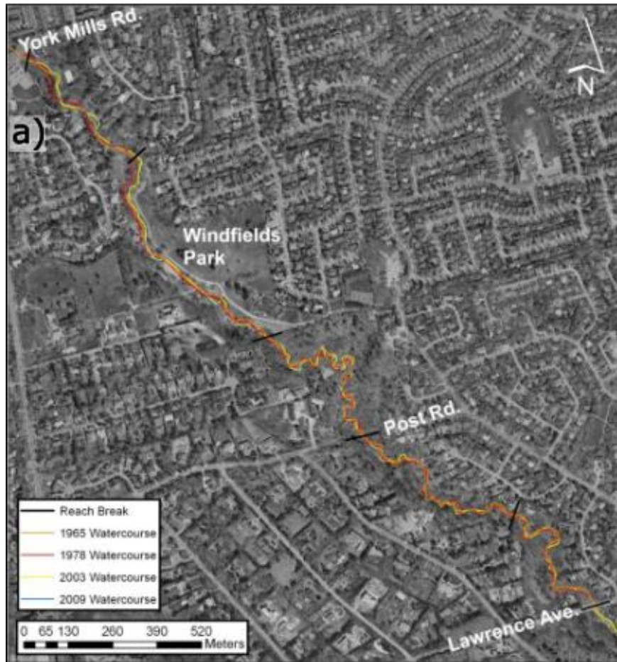
Figure 3.29: The planform alignment of a) the upstream reach and b) the downstream reach of Wilket Creek. The planform in b) begins before the beginning of urbanization while the planform in a) begins during urbanization. The greatest change in planform morphology is between 2009 and 2013. This may be due to further reconstruction after a flood event in 2005 (modified from Parish Aquatic Services, 2013).
