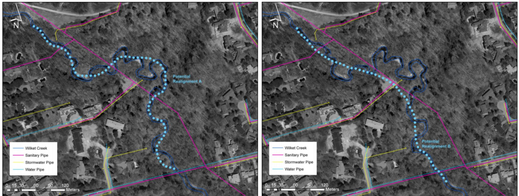
Figure 4.7: The two proposed planform designs for TRCA defined Reach 7. The high sinuosity of the channel combined with the new urbanized hydrology has led to an unstable channel; the proposed planform designs aims to stabilize this section of Wilket Creek (Toronto and Region Conservation Authority & City of Toronto, 2013).
