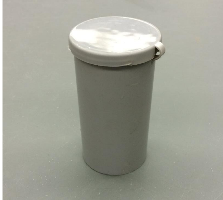
Figure 5.1 plastic cylindrical mold used in quicklime treatment
