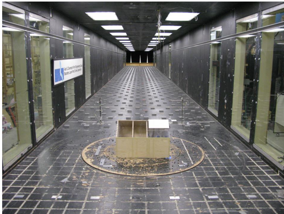
Figure 3-1: Photo of the Boundary Layer Wind Tunnel at the University of Western Ontario along with the study model having solar panels on the sloped roof (Stenabaugh, 2015).
