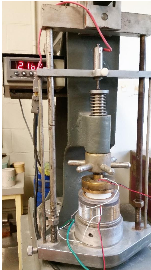
Figure 3.6. Piezoelectric ring actuator incorporated in an oedometer. A LVDT is used to track changes in sample's height.
