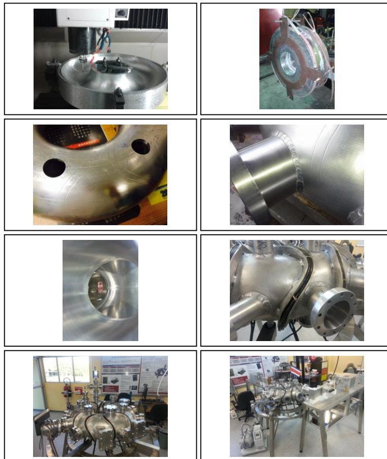
Figure 2. Stages of the vacuum vessel construction.
