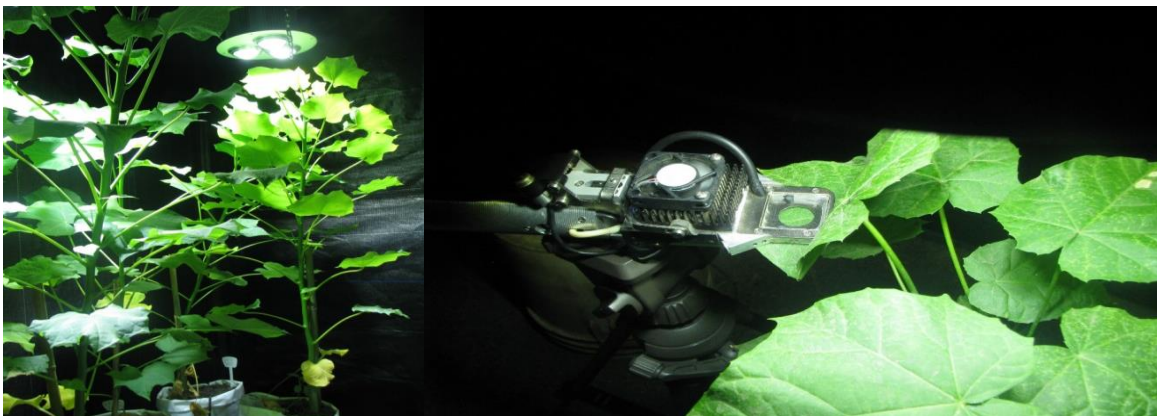
Figure 2: Growth and measurement of photosynthesis within cubicles, under selected LED bell lamp.
