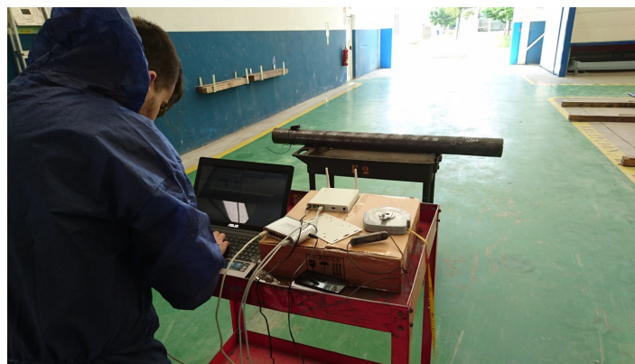
Figure 6.22: Measurements with the active UHF reader.
