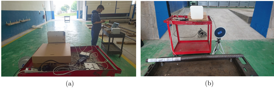
Figure 6.10: Measurements with passive UHF reader with two antennas. (a) At 17 meters; (b) At 2 meters.
