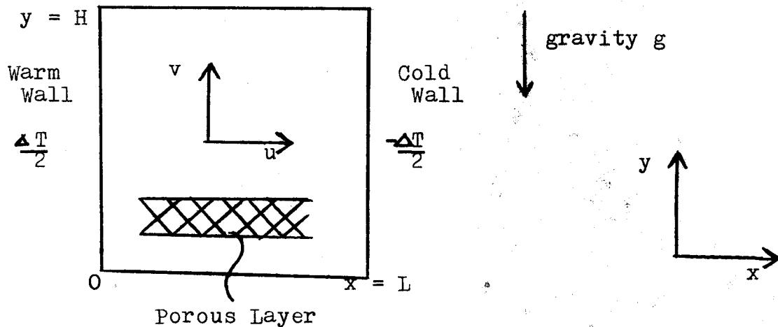
Let  $u$  denote the velocity of the fluid in the  $x$ -direction, and let  $v$  denote the velocity of the fluid in the  $y$ -direction. Let  $g$  denote gravity, which is directed in the  $-y$ -direction.
