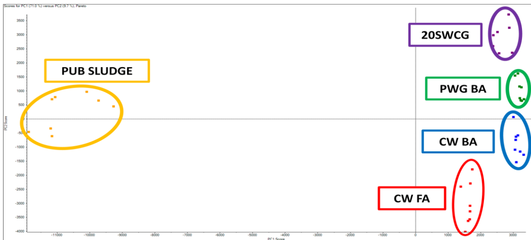
Figure 4.17 PCA score plot (A) Positive mode and (B) Negative mode, showing the relationship between the different leachate samples. The LC-QTOF-MS data in both modes were normalized and pareto-scaled prior to PCA.
