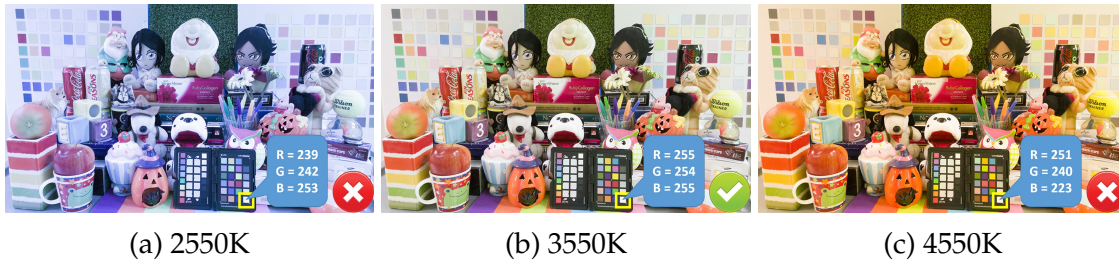
Figure 1.1: An example showing the effect of simulating different illuminations on an image. The values below images indicate illuminant temperatures in Kelvin. On the images, the RGB values of a white pixel are indicated, ideally the values should be such that R = G = B if the image is correctly white-balanced.
