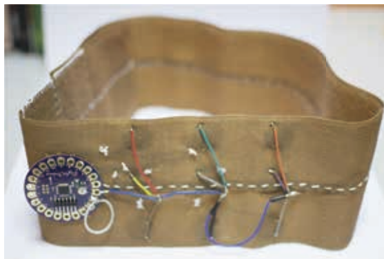
(b) The wearable Velcro Belt with 9 vibrating actuators and a Lilypad micro-controller.
