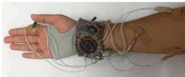
(b) Actuators are taped to the skin, and connected to the micro-controller. The button is visible between the thumb and index finger.
