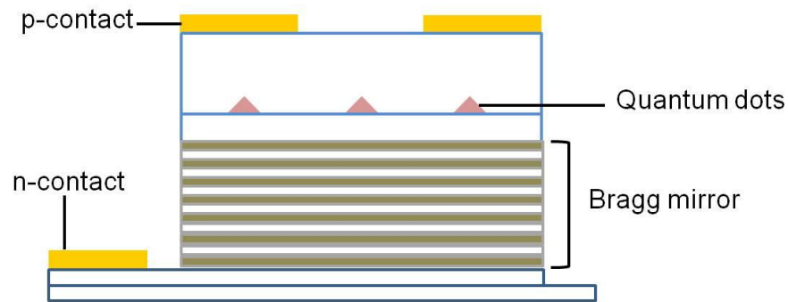
Figure 4-5. Single-photon emitter structure based on self-assembled quantum dots with electrical pumping. (Yuan et al. , 2002)
