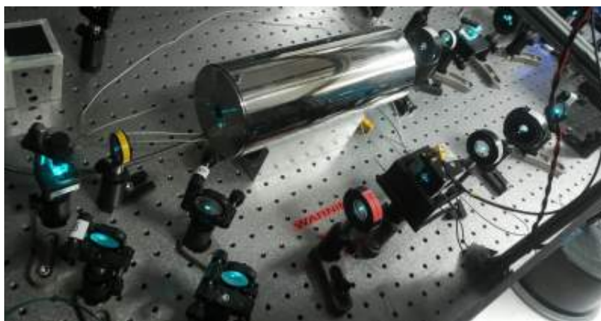
Figure 4.3: The complete tellurium cell setup. The stainless steel cylinder houses the cell. The cell temperature is 550^{\circ}\text{C} while the temperature outside the cylinder is about 50^{\circ}\text{C} .
