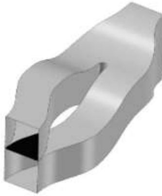
Figure 4: Illustration of a 3D micromixer with no obstructions along flow length 19
