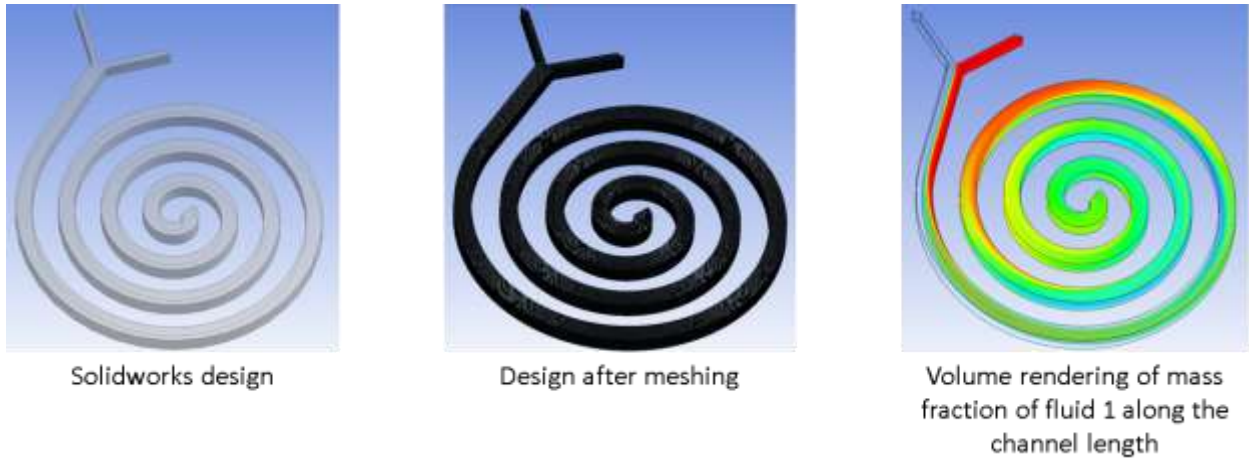
Figure 24: Illustration of the spiral design, after meshing and mass fraction of the fluid after the simulation has been completed
