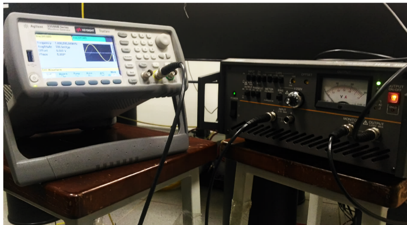
Figure 4.10 Function generator and amplifier setup.
