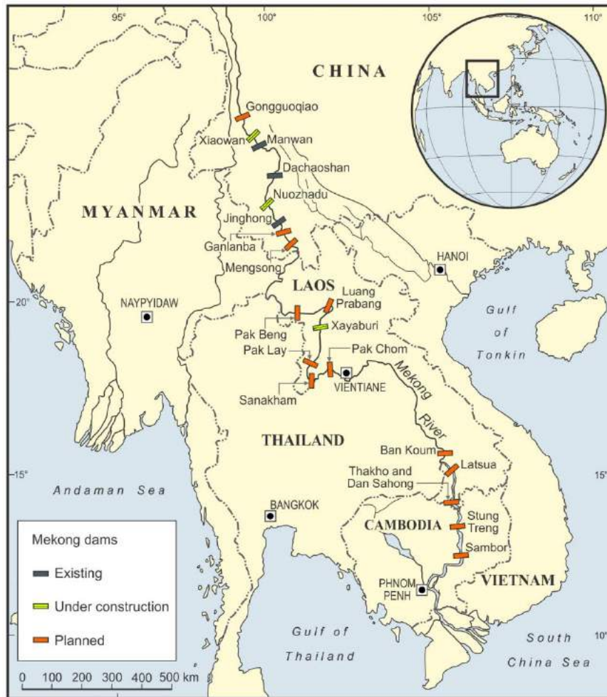
Figure 2.1: Proposed and existing dams of the Mekong river. Only dams to be constructed on the main river stem is shown. Dams that will be constructed on the tributaries are not shown (Ziegler et al., 2013) .
