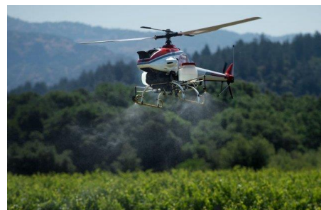
(b) UAV in spraying work
