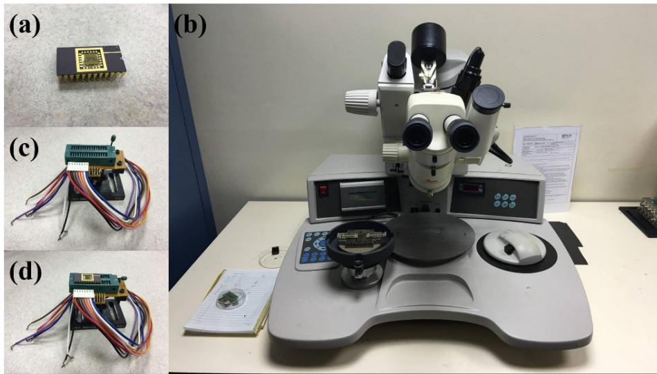
Figure 3.15 Pictures of (a) sample chip packaged with DIP, (b) wire bonder, (c) home-made socket stage with electrical connections, and (d) DIP assembled on the socket.
