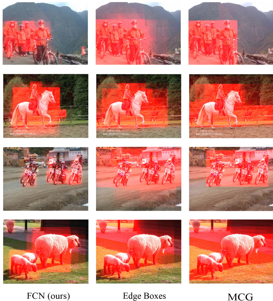
FIGURE 4.10: Examples of the proposal distribution of Edge Boxes, MCG and our method. Top 2000 proposals are illustrated for each image. For each row, our FCN is on the left, Edge Boxes is in the middle and MCG is on the right.
