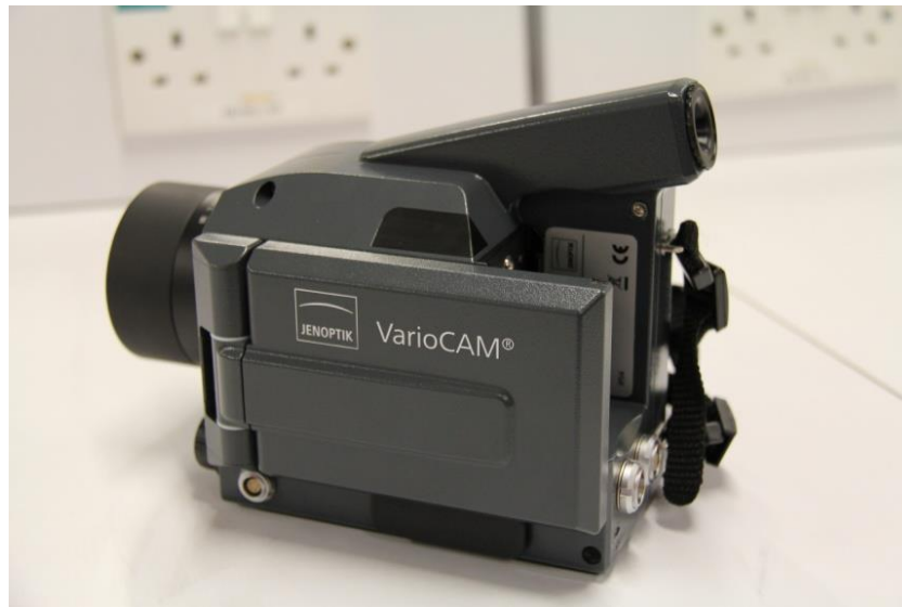
Figure 7 VarioCAM \text{\textcircled{R}} high resolution thermographic camera
