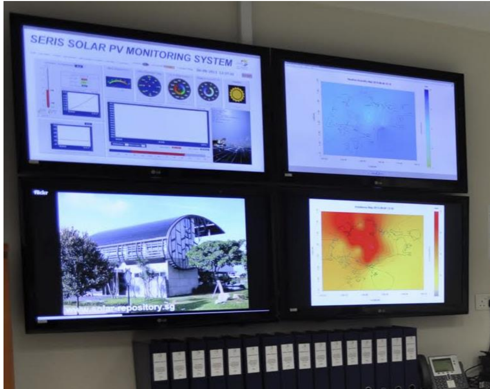
Figure 3.1.1: The PV Monitoring Lab in SERIS. A variety of meteorological parameters such as instantaneous solar irradiance level, spectrum, wind speed, ambient temperature, and real-time performance of PV systems are measured and monitored.
