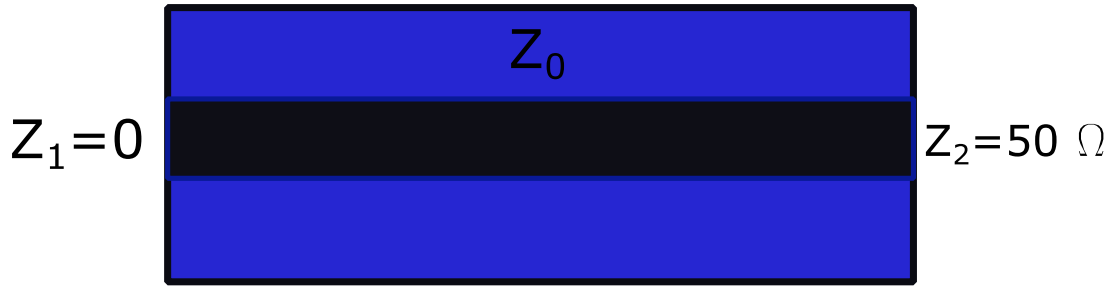
Figure 5.1 Schematic diagram of the shorted coaxial transmission line (cross-section) of characteristic impedance Z_0 , with one end shorted Z_1=0\Omega and the other end terminated with a microwave source Z_2=50\Omega .
