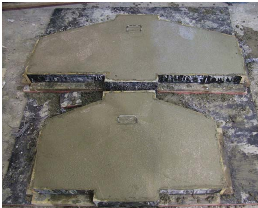
(b) Casting of corbel specimens
