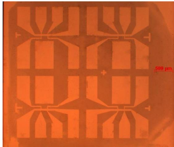
**Figure 5.2** Optical microscope image of the Hall bars patterned on a  $5 \times 5 \text{ mm}^2$  Pt/BTO/STO sample. Four Hall bars were fabricated on the  $5 \times 5 \text{ mm}^2$  sample.
