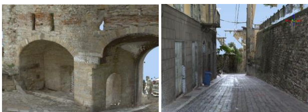
Figure 6. Two views of the point cloud acquired with the MMS in the historic city centre of Bergamo "Città Alta".
