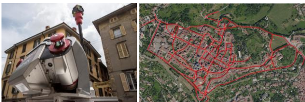
Figure 5. Configuration of the SINECO MMS (left) and the trajectory of the surveyed area (right).
