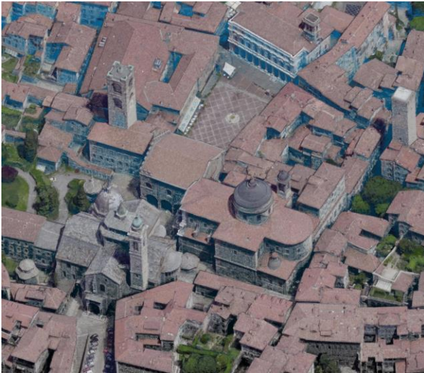
Figure 4. Close view of the shaded 3D point cloud (1 GSD resolution) of the historic centre.
