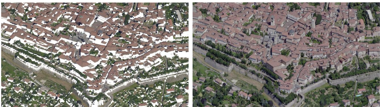
Figure 3. The same part of the historical city seen as 2.5D DSM cloud (left) and 3D point cloud (right).
