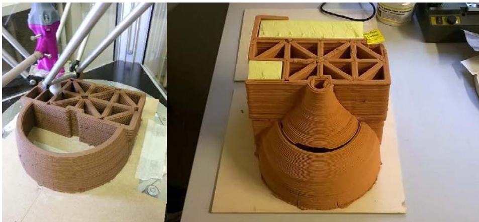
Fig 4. Clay 3D printing studies for components with specific design requirements (insulation assembly and light integration).
