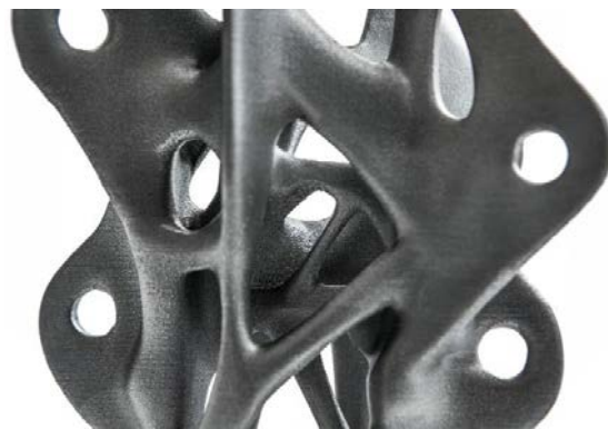
Fig 2. Arup studies on topological optimization of metal 3D printed joints.
