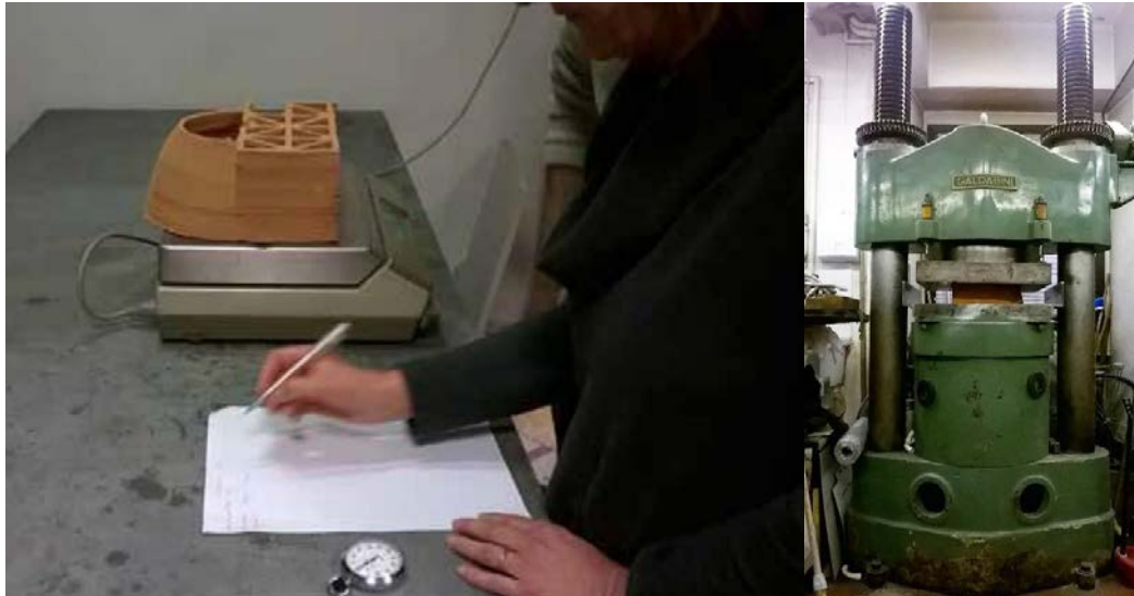
Fig 5. Absorption and structural testing of the 3D printed clay brick.
