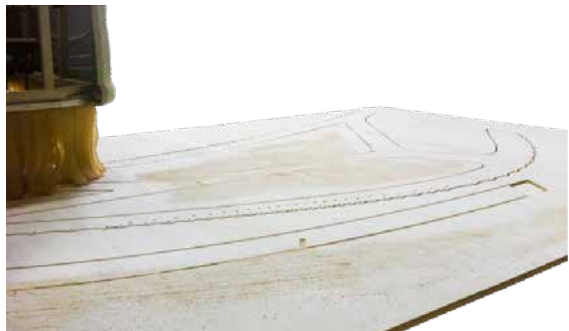
Figure 15: CNC milling of a poplar plywood vertical warp and an horizontal support
