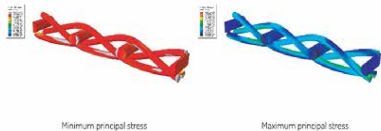
Figure 7: FEM analysis of a typical Striking & Stranding pattern and its minimum and maximum principal stresses
