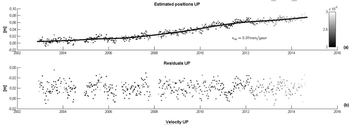
Figure 3: Thule DORIS site Up component time series plus estimated long-term signal (a) and residuals with quasi-cyclostationary behavior (b). A mean velocity  $v_m = 5.97 \text{ mm/yr}$  has been estimated as a mean value of  $\dot{p}$ .
