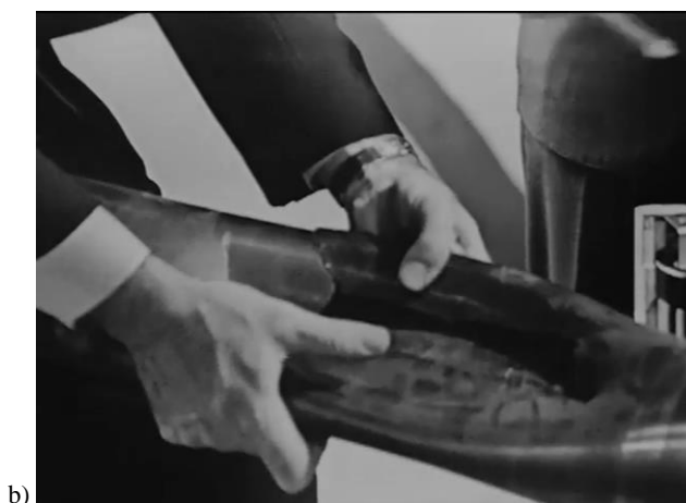
Figure 1. (a) Water density, salinity and temperature variation with depth (Ocean Stanford Edu). (b) Effect of pressure at high depth: Steel waterproof camera housing collapsed at a depth of about 6000 m (frame extracted from EDC).
