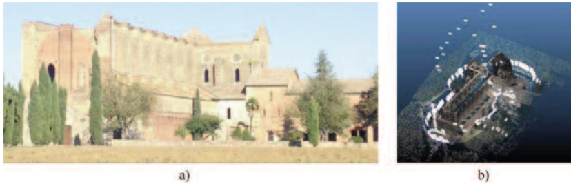
Figure 3. The Abbey of San Galgano close to Siena, Italy. (a) The imaging network (ca 200 images) for the surveying of the complete Abbey (b).
