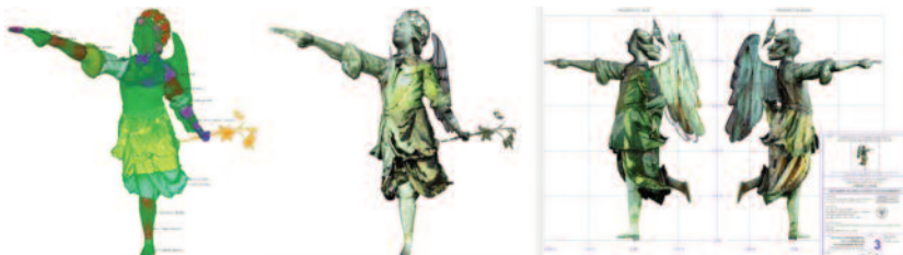
Figure 8. View of the segmented point cloud of the statue (left), the produced polygonal textured model (middle) and the 1:10 representations for restoration purposes (right).
