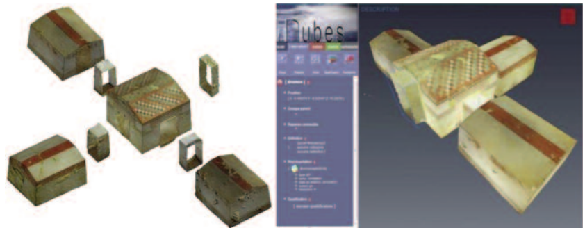
Figure 6. The produced and exploded 3D model of the heritage structure (left) and its visualization in the NUBES platform (right).
