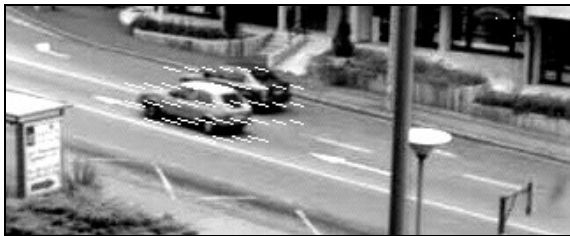
Figure 6. Motion detection using optical flow.
