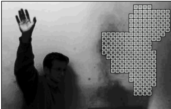
Figure 5. Snapshot of the detection alarm. The non-smoke motion is not detected.
