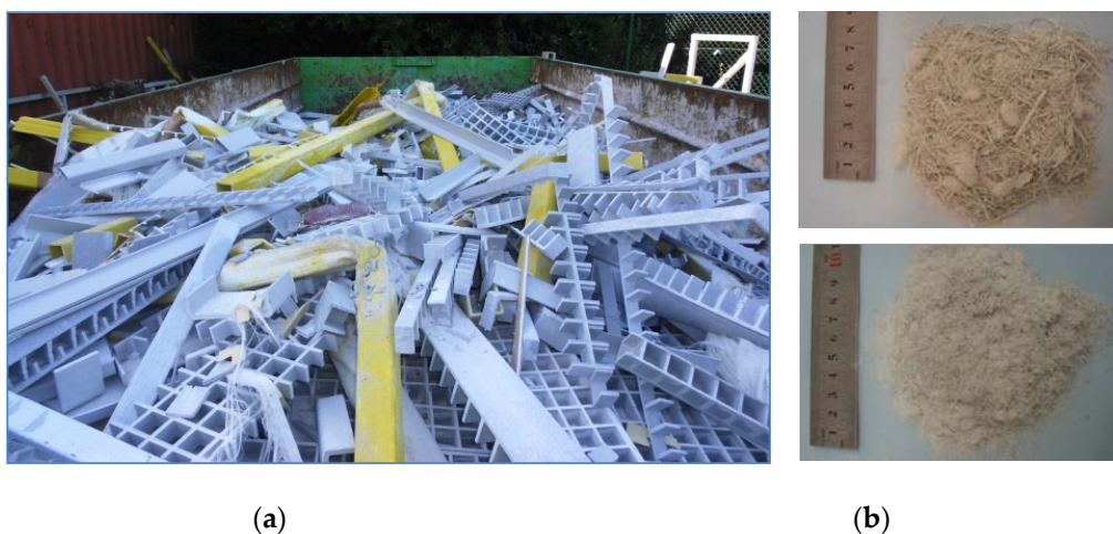
Figure 3. (a) typical waste of GFRP pultrusion process; (b) samples of obtained recyclates after mechanical recycling in a heavy-duty cutting mill using different sized-meshes inside the grinding chamber.
