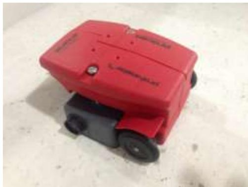
Figura 5.4 – Sonda Universal e ScanCar – PROFOMETER 5+
