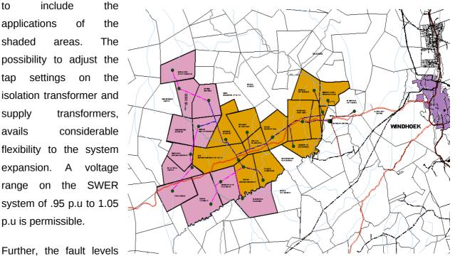
Geographical arrangement for a rural farmers SWER scheme were marginally low. For a SWER system, fault levels of 50A to 70A can be manageable from a protection coordination point of view. Protection and fuse grading would be a separate exercise to be
