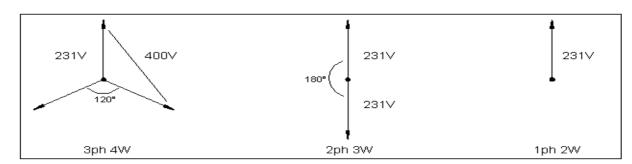
Figure 4: Schematic – Phase arrangement [3]
