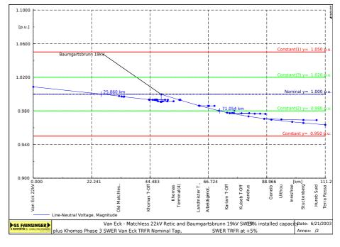
Load flow simulation results - Voltage profile
