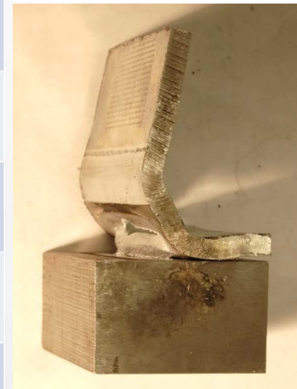
Peel strength > 250 N/mm
