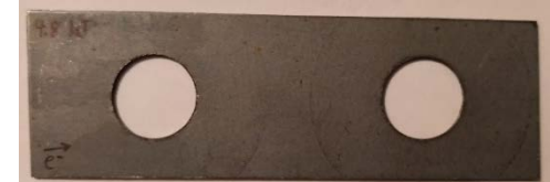
1.5 mm thick 1500 MPa boron steel
