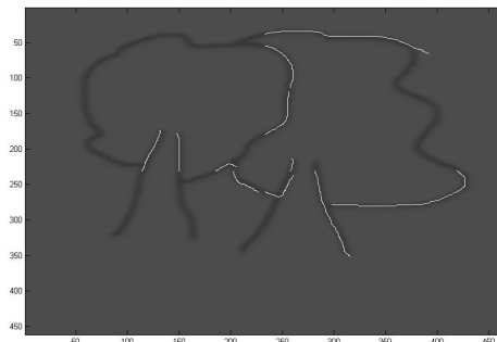
Figure 2: Illustrating the tracking paths generated by the EKF. White line segments indicate the tracked path, whilst the darker lines indicate the image line strokes. This example shows the tracking of 11 segments.
