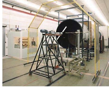
Figure 2 – The model wind turbine and open jet wind tunnel used
