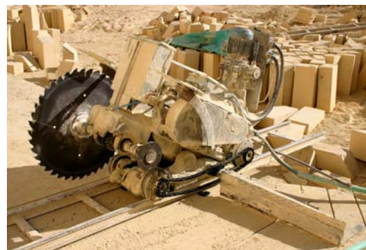
Figure 2. Typical cutting machines as used in softstone quarrying: (a) machine used to make horizontal cuts through bedrock and (b) machine used for vertical cuts.
