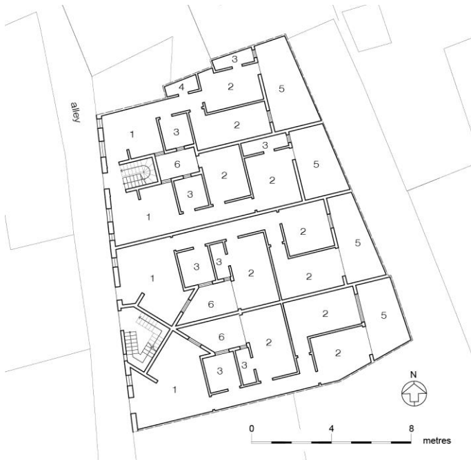
Figure 9. Internal layout: 1) kitchen/dining/living room, 2) bedroom, 3) bathroom/shower, 4) store, 5) back garden, and 6) internal yard.
