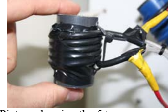
Fig.7. Picture showing the 5 turn coax sensor used
