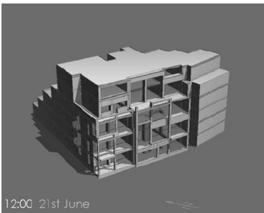
Fig 8. A Figure of the Summer shading analysis of the concrete screen shaded apartments
