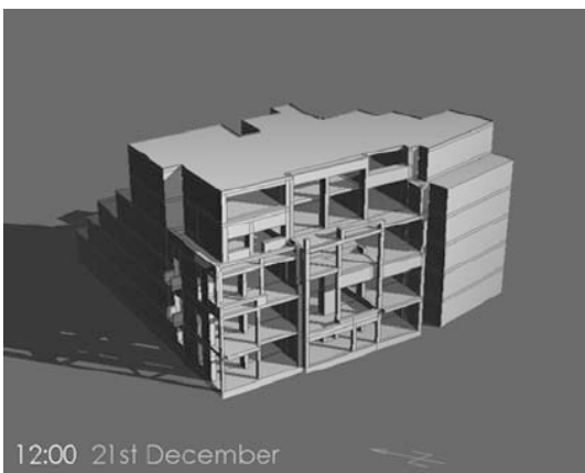
Fig 9. A Figure of the Winter shading analysis illustrating the shallow winter sun in Malta
