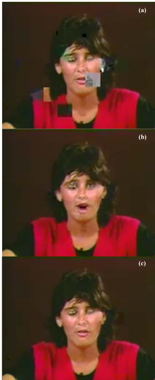
Fig. 6 Miss-America using (a) MB level concealment, (b) Slice Level Concealment, and (c) Proposed Error Detection method
