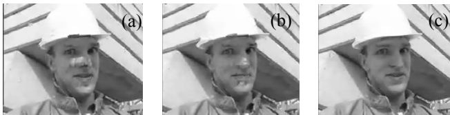
Fig. 3 Frame 202 for the Foreman sequence (a) Syntax Analysis method (27.00dB), (b) Standard Decoding (27.60dB), and (c) proposed solution (33.23dB).
