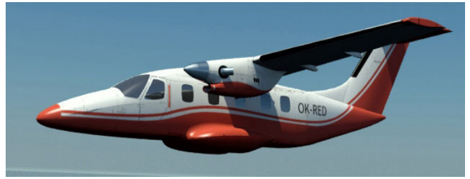
Figure 7: Evektor EV-55 business jet [37], as included in the electromagnetic propagation simulation.
