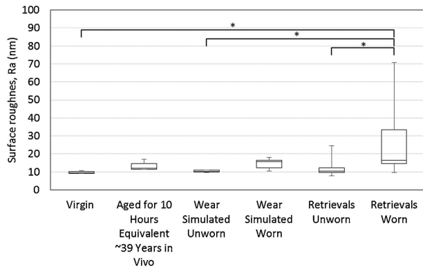
Figure 9. Comparison of Surface roughness across all groups. A significant difference in surface roughness [ F(5,57)=5.05 , p=0.001 ] was found. In contrast to the average V_m , the post hoc tests showed the significant difference to be between the R_a of the worn area of the retrievals and the virgin and aged samples with no difference between the unworn area of retrievals and the surface roughness of the virgin, artificially aged, or wear simulated heads being observed.
