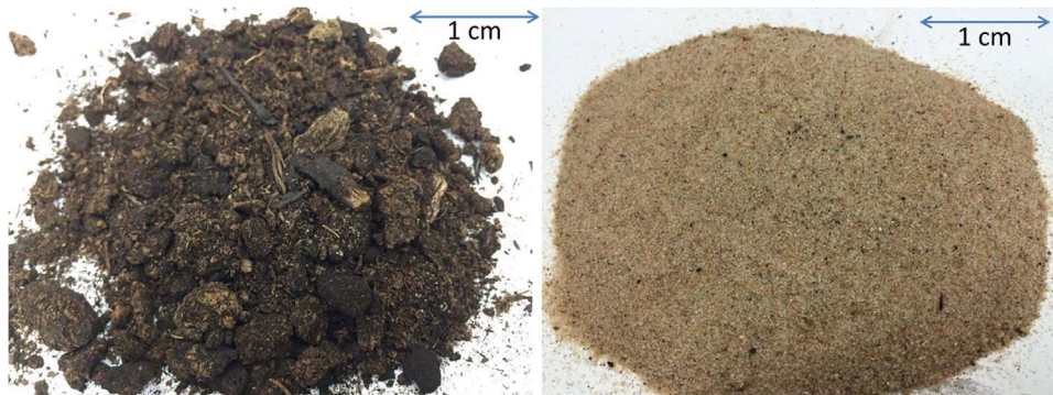
Fig. 3. Peat (left) and sand (right) are mixed to create the appropriate inorganic content ratios of our samples.
