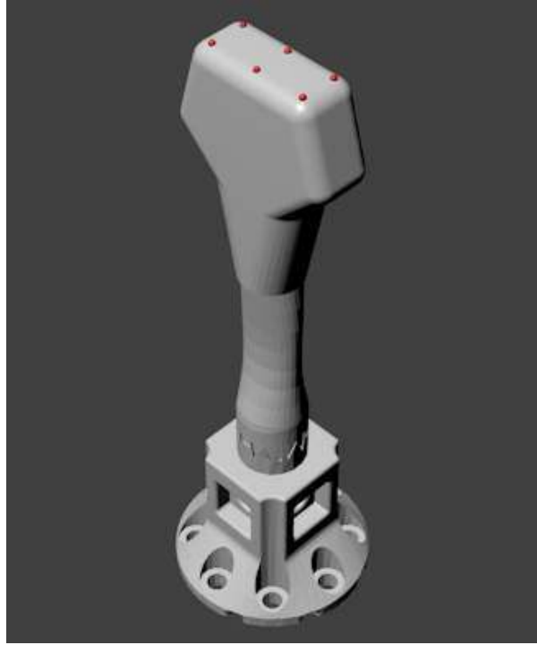
Figure 6.9: Rendering of the US probe tool with the points used in the closest point search for computing body feedback in red.
