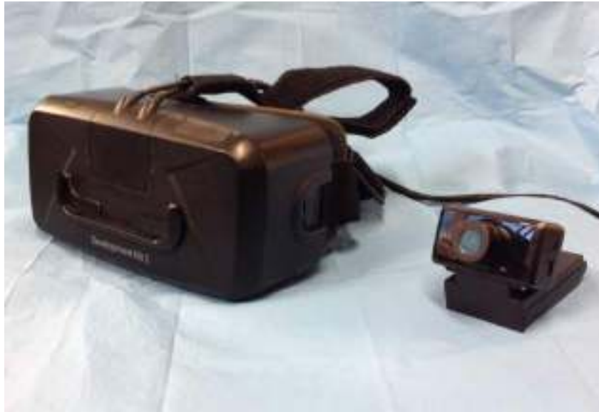
Figure 6.5: The Oculus Rift head-mounted display and tracking camera.
