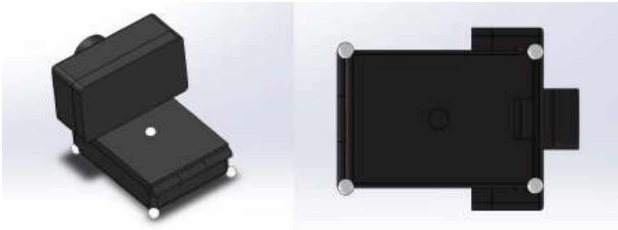
Figure 6.7: Oculus Rift tracking camera with the points touched highlighted with spheres.
