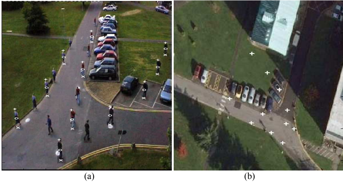
Figure 5. The verification of homography estimation for multiple parallel planes: (a) an individual camera view and (b) the top view from Google maps. The feet of the pedestrians in (a) are manually localized and projected to (b) through the ground-plane homography. Then they are back projected to (a) through homography induced by planar planes parallel to the ground plane.
