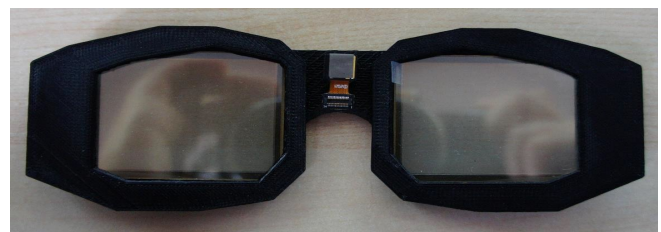
Figure 7. Final prototype frame with on-board webcam, improved nose bridge and frame curved by 15° for a more natural wearing experience
