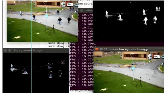
Figure 4. \mu TOLED-20-G2 in frame Version Object detection software running on CPU with average FPS @ approx. 10.6
